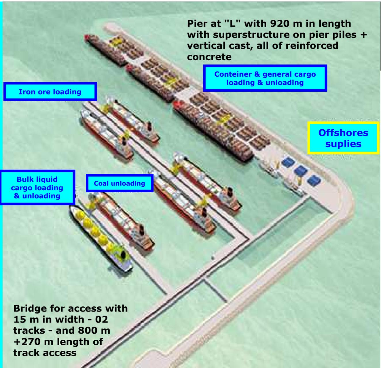
Bridge for access with 15 m in width - 02 tracks - and 800 m +270 m length of track access
